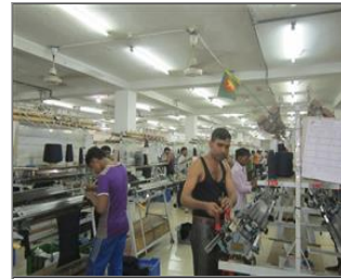
Photo of non-conformity Workers not using face mask at knitting section.JPG
